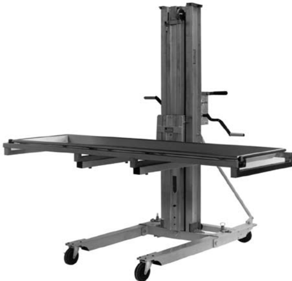
Transfer from Cadaver lift to Autopsy Carrier
